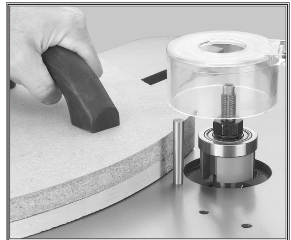
Figure 35. Hold-down jig used to support workpiece.
